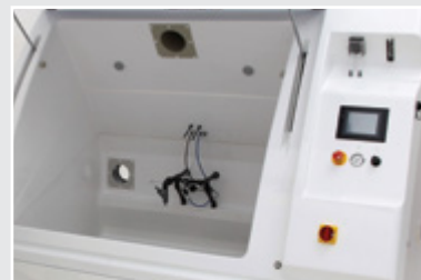
3 The Atmosfär chamber is now ready for other types of corrosion test.
